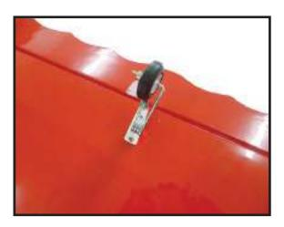
3) Hold the rudder in place and mark it where the music wire will enter. When you are happy with the fit, fill the hole with epoxy and use CA to glue in the rudder hinges.
