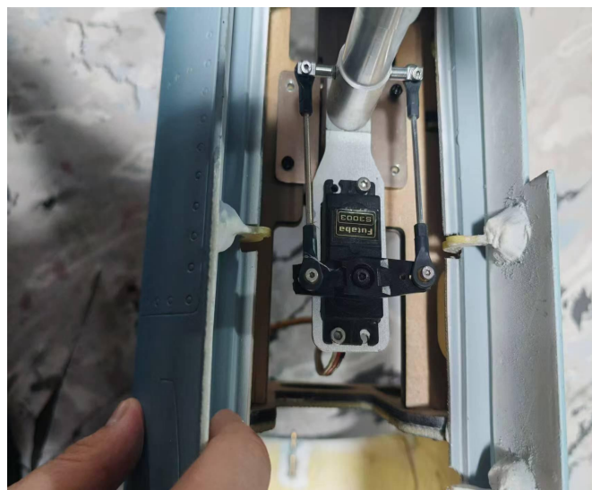
27 more picture about the installation of front retract
