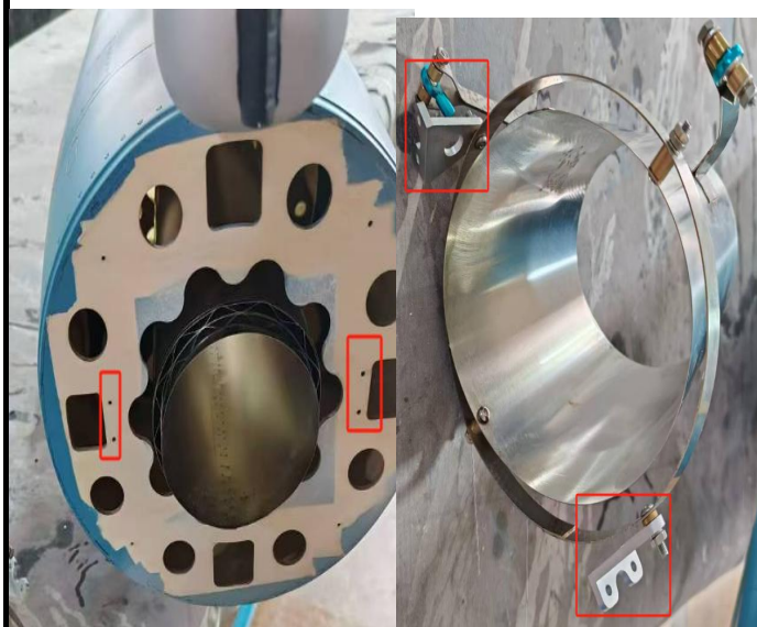
33 Connect the carbon fiber push rob with the vector and servo
