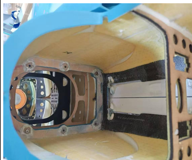
30 Fix the front fuselage via installation screws hole
