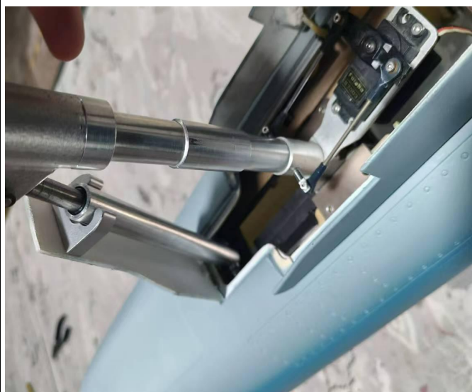
26 fix the front retract with screws as the picture
