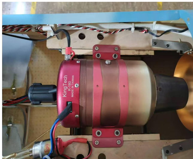
38 The pictures about the turbine installation
