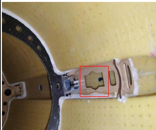
35 More picture about the rudder servo installation
