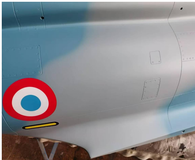
37 Lock the rudder via the two holes in the picture
