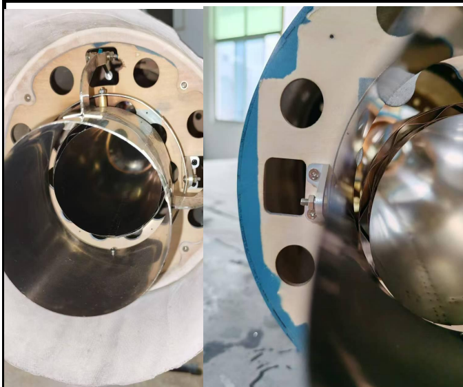
33 Connect the carbon fiber push rob with the vector and servo
