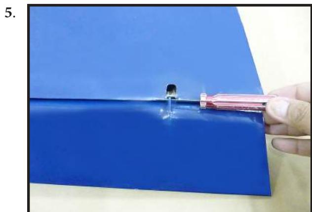
Attach the flap linkage to the control horn. Slide the clevis retainer over the forks of the clevis.
