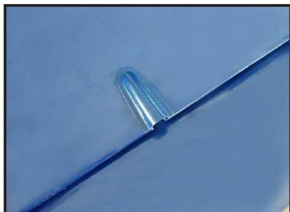
Use canopy glue to attach the cover to the wing. Use low-tack tape to keep the cover in position until the adhesive fully cures.
