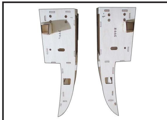
You install the side motor mount box with the lettering 399L on the left wing and 399R on the right wing.
