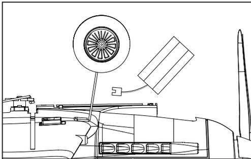
3. Connect the battery to the receiver and insert the battery into the battery box. Then, place the battery wires inside and close the battery box door.
