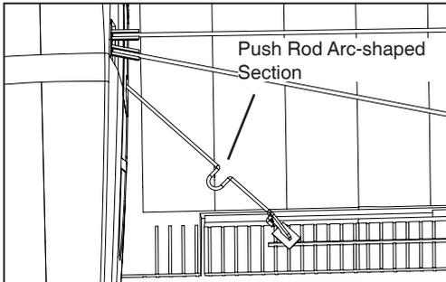
If the aileron is not properly centered, adjust the push rod length by bending the arc-shaped section slightly with needle nose pliers until the aileron is centered.
