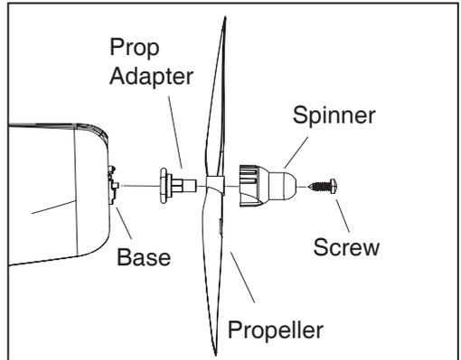
Follow these steps to replace a broken propeller and/or prop adaptor. You will need a Phillips screwdriver and needle nose pliers (not included).
