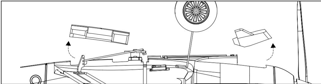
The control board and motor can be accessed by removing the hatches on the bottom of the fuselage. No tools are required. Gently pry the hatch open with your fingers.
