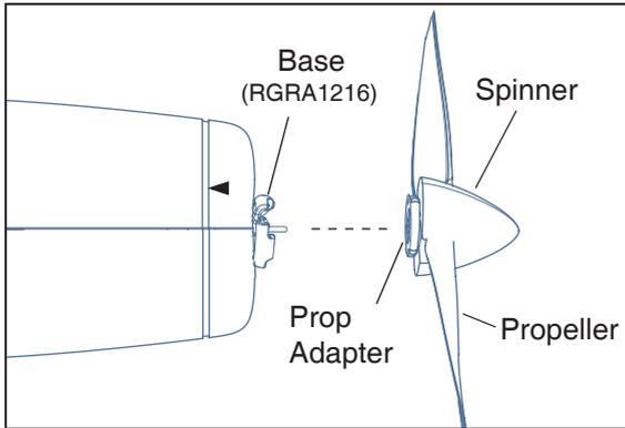
Each Prop/Spinner set includes the propeller, spinner and prop adapter.
