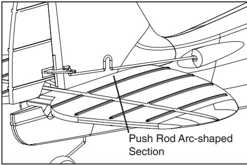
If the rudder is not properly centered, adjust the push rod length by bending the arc-shaped section slightly with needle nose pliers until the rudder is centered.
