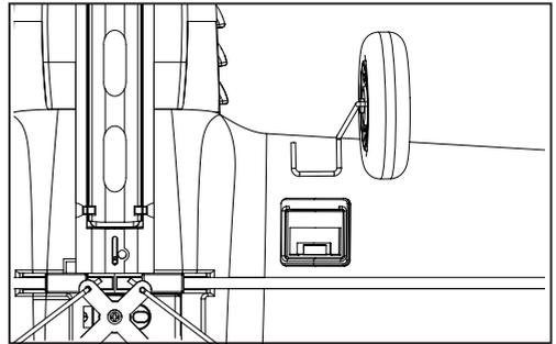
2. Plug the landing gear into the wings as shown above, press until gear clicks into place.
