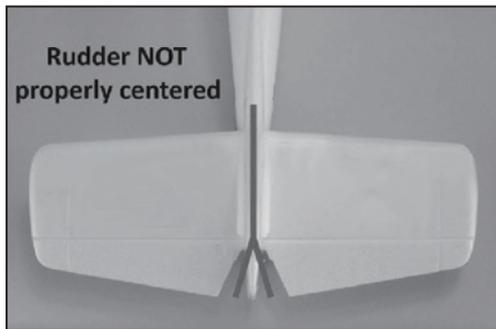
Check that the rudder is properly centered as shown above.
