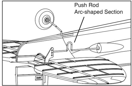
If the elevator is not properly centered, adjust the push rod length by bending the arc-shaped section slightly with needle nose pliers until the elevator is centered.
